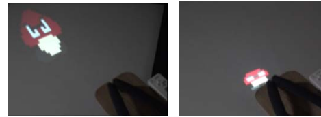
Figure 3: The graphic changes depending on the proximity of the shoe-shaped I/O interface.
