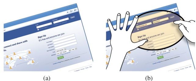
Figure 3: (a) A protected web page requiring login. (b) Moving the lens over the login area automatically fills in credentials and enables login by simple touch.
