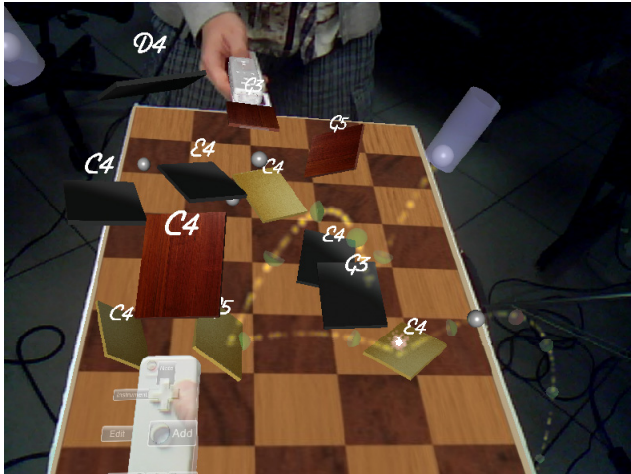
Figure 1. Two players ready to add bars to the environment. (Tracked Wii remote controllers, and parts of players' hands are visible because occluding geometric models of the remote controllers are added to the scene.)
