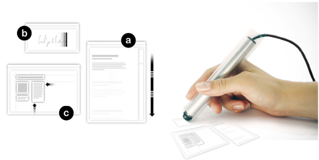
Fig. 1.: Stylus and GUI, displaying stickiness-augmented newsreader (a), resistive signature field (b) and rubberized grid lines (c).
