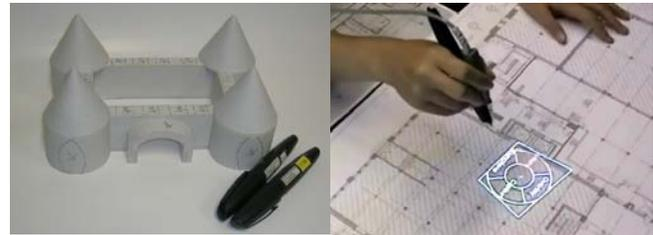
Figure 1 (a) The ModelCraft system can capture annotations and edit marks on the surface of 3D models. (b) PenLight system dynamically overlays digital information on top of a physical printout.
