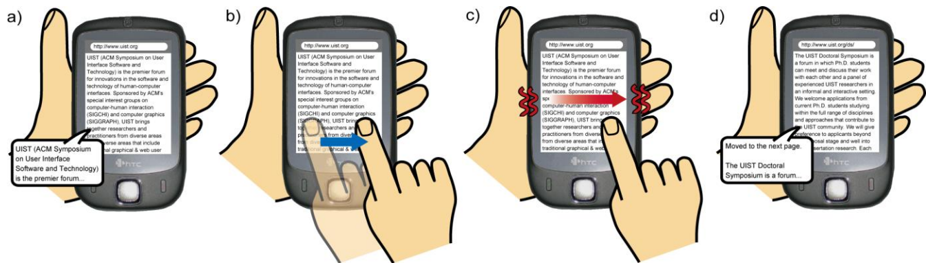
Figure 3. Use of peripheral tactile feedback for hand gestures on the screen: a) A web browser application; b) The user performs a swipe gesture from left to right on the screen; c) The system provides tactile feedback corresponding to the gesture that the user is performing (in this case, a vibration pattern from left to right). This allows the user to know whether she is performing her intended gesture correctly; d) After the user releases her finger, the system executes the command associated with the gesture (in this case, moving to the next page).
