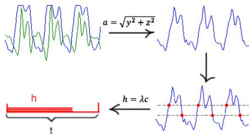
Figure 2: Algorithm of calculating running time.
