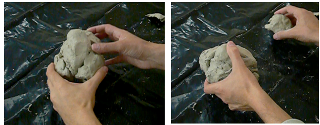
Figure 1. Left: interacting with a model composed of 6 sensors. Right: additive and subtractive modeling is supported. Here a piece of clay containing one sensor is removed.
