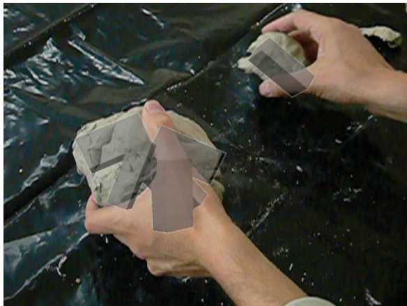
Figure 3: Sensor data (left) and corresponding isosurface (right) overlays on video image of sensors. (Registration of the images was done by hand, but all relative position & orientation is computed from the sensor data)
