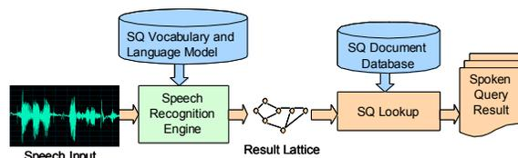
Figure 1: The speech recognizer's result lattice is used to create a query term vector that is compared against the document feature vectors.
