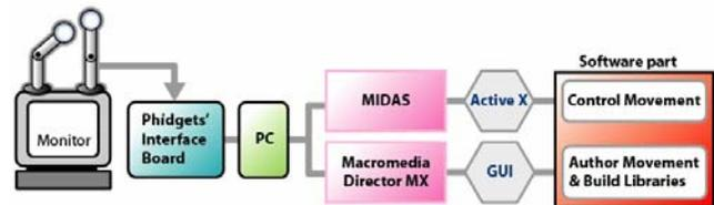
Figure 3: The infrastructure of hardware and software.
