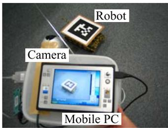
Figure 1: A prototype version of Shepherd
