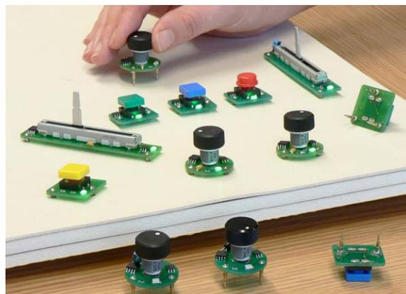
Figure 2: The VoodooIO architecture: substrate material and control devices.
