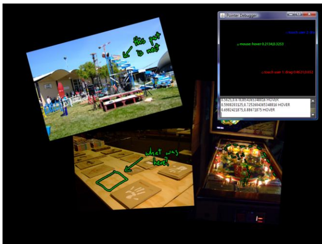
Figure 2: Photo tagging application we developed using the Pointer API. Users can move pictures with their hands and annotate them with a pen. Inset: the debug sidebar.
