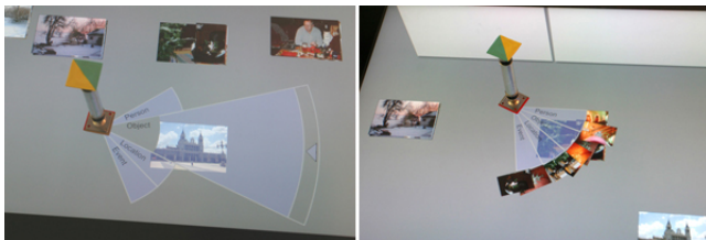
Figure 1: Screenshots from the Living-Room project [7] Left: Annotating pictures. The extended region can be used for (hand) writing in annotations. Right: Filtering the images of one pile. Previews of matching photos are shown on the outskirts of the semi-transparent overlay.
