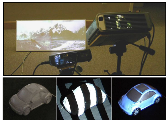
Figure 3. Multi-projector stitching ( top ) and appearance augmentation of 3D objects ( bottom ).
