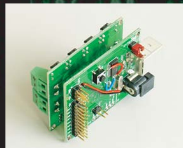
The control unit consists of a microprocessor, a USB controller chip and an H-Bridge.
