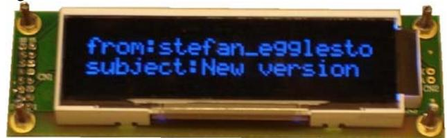
Figure 1 –PhidgetTextLCD device
