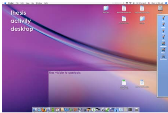
Figure 3: An initial (non-interactive) prototype of the Giornata user interface. Notable features are the presence of free-form activity tags ( upper left ), files specific to the activity and spatially grouped to indicate public or visible to contacts status, and a streamlined sharing palette interface ( right ).
