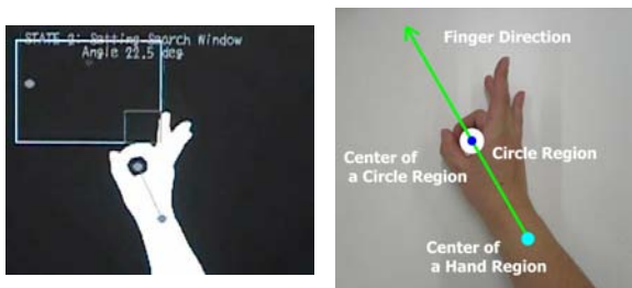
Figure 3: Left: Circle region and search window position. The window is set to the position that moving finger passes through its inside. Right: Flicking angle is based on the position of circle and hand region, or a virtual marble and circle position.
