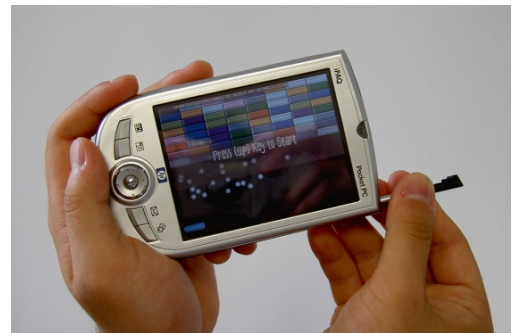
Figure 1: An interaction style of RodDirect; A user rotates and slides the stylus to operate handhelds.
