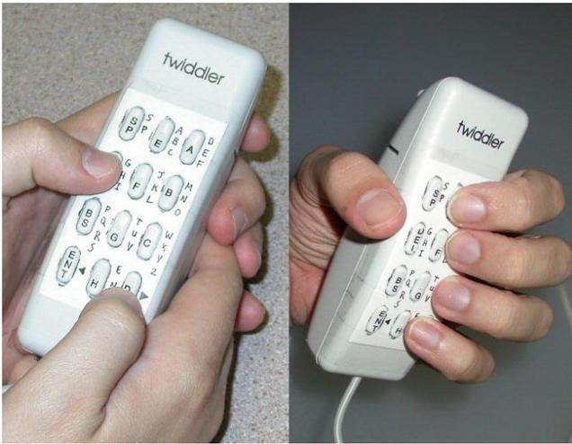
Figure 1: On the left, typing using multi-tap on the Twiddler keypad. On the right, chording with the Twiddler one-handed keyboard typing the letter 's'.
