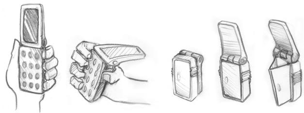
Figure 5: A mobile phone design which incorporates chording capabilities.
